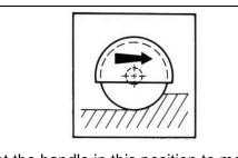
Set the handle in this position to move the machine forwards
