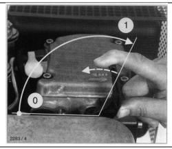
Turn the decompression lever until stop "1" is reached. In this position you can hear the automatic decompression system engage.
