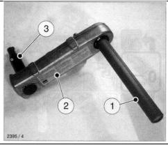
You must hold the tubular grip firmly to maintain contact all the time between the starting handle and the engine. Maintain turning force during the entire hand starting operation.
