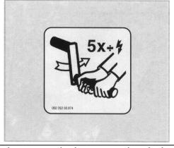
After the automatic decompression device has engaged at its limit stop, turn the crank five times to build up compression.
