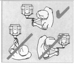
Position yourself on the side of the machine, following the drawing. Always hold the tubular grip with both hands. Turn the handle slowly until the pawl engages in the ratchet, then increase turning force to build up speed. The highest speed must be reached when the decompression lever returns to the "0" position. As soon as the engine has started, pull the starting handle out of the guide sleeve.
