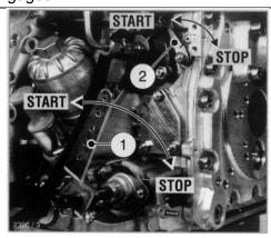
Set the control lever "1" to a position between ½ START and max. START, according to requirements. Selecting a lower engine speed will reduce smoke when starting.
