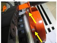
• To be able to use your machine, you must release the head of cut. For that unscrew the knurled button which maintains the head on the right amount during transport.
