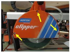
• Loosen the hexagonal nut (left threaded) on the blade shaft using the 18 mm wrench supplied with TR 202, which holds the removable outer flange.
