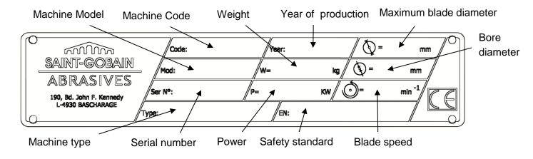
Important data can be found on the following plate located on the machine:
