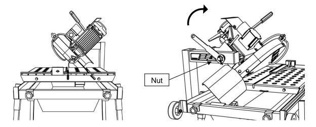
With the CM~43 it is possible to make fixed or multiple step bevel cuts.
