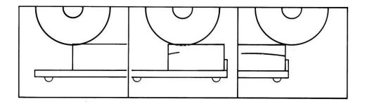
Multiple step cutting consists of moving the conveyor cart with the material to be cut back and forward under the rotating blade,
