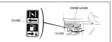
Move the choke lever to the CLOSED position.
