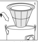
• Mount the head on the drum and secure it with the hooks
