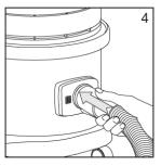
• At the end of the hose, insert the handle and extensions. Choose and connect the most suitable accessory.
