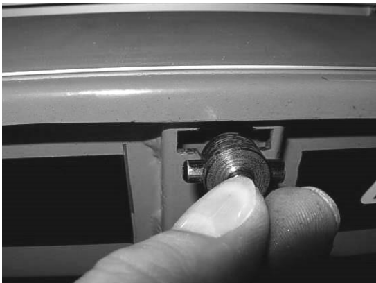
Insert 2 threaded and pinned shafts
