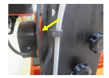
• Mount the pump in the vat to water and the drain plug
