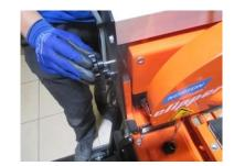
· Tighten angular cutting guide
