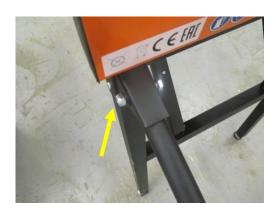
• To be able to use your machine, you must release the head of cut. For that unscrew the knurled button which maintains the head on the right amount during transport.
