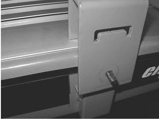
Insert both guide supports and lock them with knobs
