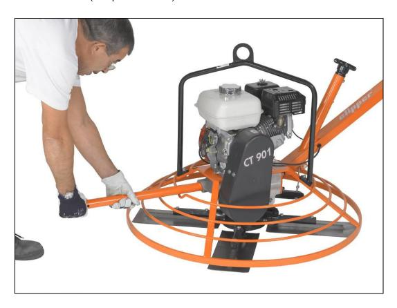
To lift the machine, use the lifting eye. Make sure that your lifting device is securely fastened to the lifting eye.
