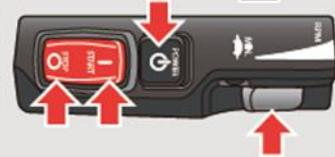
**2 LED** Check all LED light ON when POWER is turned on
