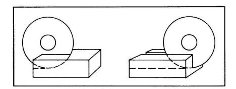
In full depth or fixed cutting, the cutting head is locked in a fixed position and the material is pushed into it as shown.
