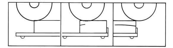
Multiple step cutting consists of moving the conveyor cart with the material to be cut back and forward under the rotating blade,
