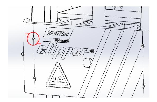
Screw gently the M8 screw by 1/8 of a turn to adjust the slider' clearance.
