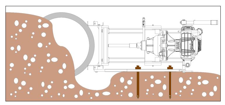
Place the machine on the ground, perpendicular to the pipe axis, fix it with the two peak of anchorage, so that the base of the tube adheres well to the pipe with its two points of support (centering effect).
