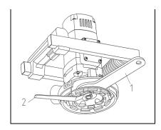
First of all, the detachable hood segment has to be removed. The snap fit opens up and the segment is pushed forward. Now you can hold up the driving disc between gearbox and grinding wheel by using a jaw wrench 32 (1). Use the face spanner (2) to unscrew the driving nut. Then remove the mounted grinding wheel respectively mount the new one. The assembly works the other way round!
