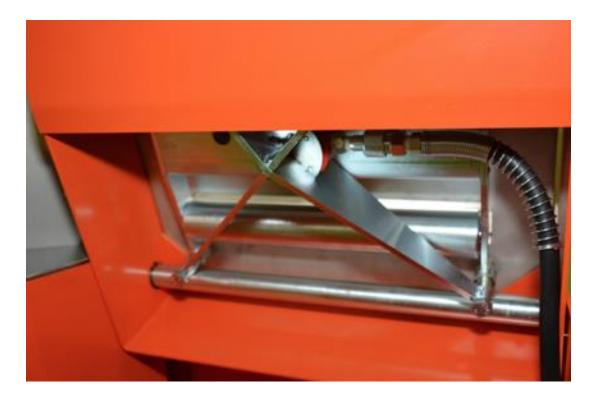
Step 6.: Finish the assembling of the roller table kit with tightening of the table screws. Now, you may continue with the placement of the bloc according to the point 5.2.1 Preparing the cut with roller table. Caution: The manual hydraulic pump has an integrated pressure limiter what means you may use the manual hydraulic pump as long as the rollers reach the final position ... if, you continue with pumping the hydraulic pump the hydraulic system is secured any time!
