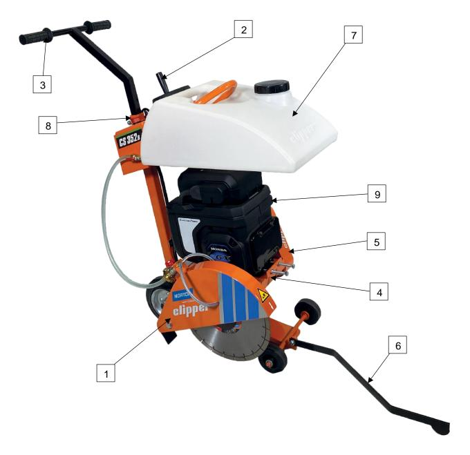
Made of jig welded open profile steel, the **CS 352** is stable but at the same time, easily transportable.
