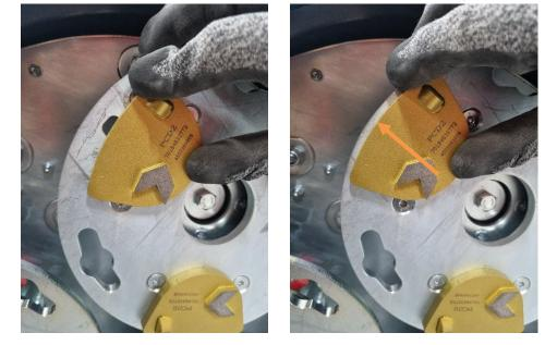
• Slide the tool into the hole from the center to the outside of the tool tray until it locks.
