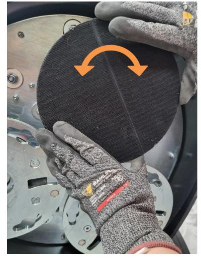
• Turn the support plate in the opposite direction of rotation to lock it
