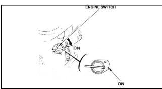
Move the throttle control lever slightly to the left. Put the engine switch on ON.
