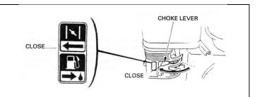
Move the choke lever to the CLOSED position.
