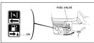
Turn the fuel valve to the ON position. Fully press the dead-man handle against the main handle.
