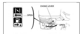
As the engine warms up, gradually move the choke lever to the OPEN position.
