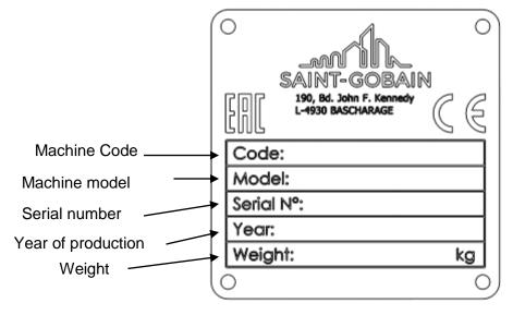
Important data can be found on the following plate located on the machine:
