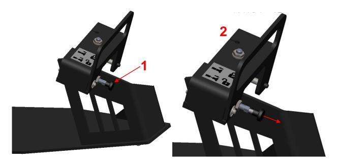
• While pulling the button, pivot the part (2) thanks to the handle (3).
