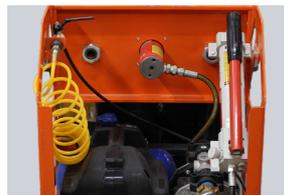
HYDRAULIC PUMP WITH PRESSURE VALVE
