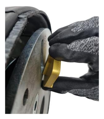
• Slide the tool into the hole from the centre to the outside of the tool support until it locks.
