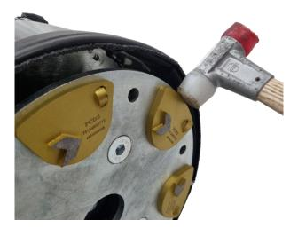
Place the tools by positioning the dovetail of each tool in the inner part of the fixing hole. A
