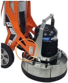
• Adjust the head position according to the floor to be treated
