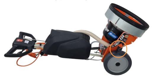
• To set up the support, simply center it on the head of the machine and make a slight rotation to lock it.
