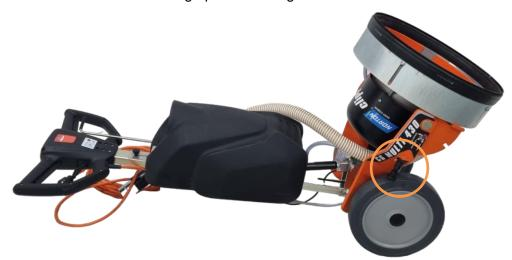
• Simply center the brush on the head of the machine and make a slight rotation to lock it.
