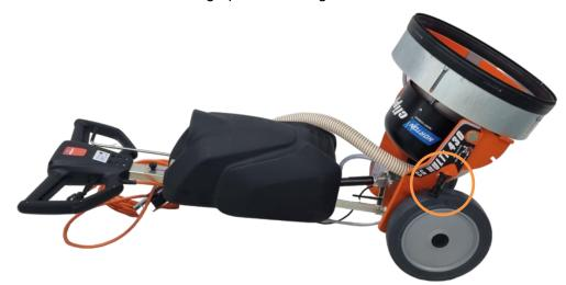
Center the planetary on the head of the machine (taking care to set up the gears) and make a slight rotation to lock it.
