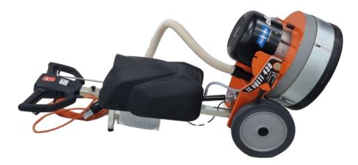
• Lock the head in the tool change position using the indexers.
