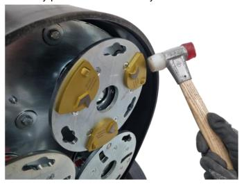
• Place the tools by positioning the dovetail of each tool in the inner part of the fixing hole. A magnet holds each wing before it is locked.
