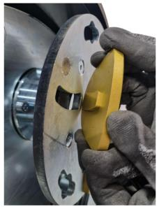
• Slide the tool into the hole from the center to the outside of the tool tray until it locks.
