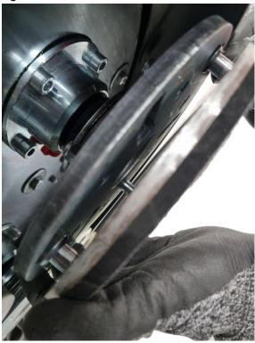
• Turn the support plate in the opposite direction of rotation to lock it
