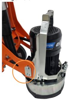
Adjust the head position according to the floor to be treated
