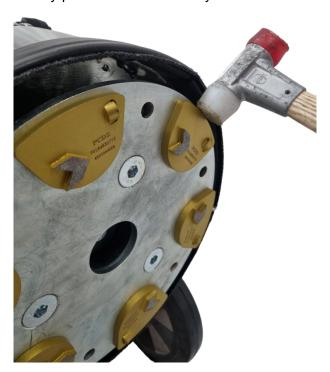
Place the tools by positioning the dovetail of each tool in the inner part of the fixing hole. A
