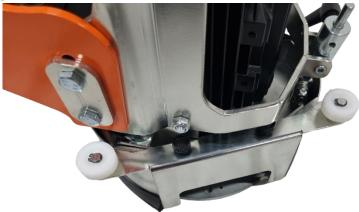
Align the wheels with the wall guide by lifting the handle and rotating the wheels.
