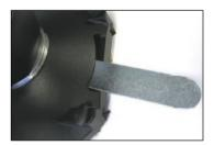
Through the opening at the protection cover now you can hold up the driving disc between gearbox and grinding wheel by using the jaw wrench 32 included in the delivery.
